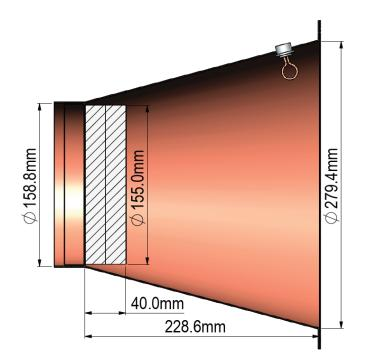
The SPR design spreadsheet, described in our IAC-20 paper, was used to calculate the resonant frequency at the interface axial length of 188.6mm using TM012 mode. (Note the loop orientation is for TM modes)
