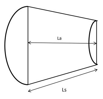
For flat end plates Path length error = Ls-La Total error =Q(Ls-La) leads to wavefront phase error and reduction of Q End plates must be shaped and aligned to minimise mean path length error.
