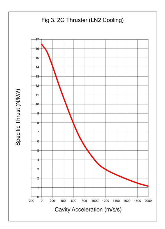
Superconducting second generation thrusters were then modelled, cooled first with liquid nitrogen and then with liquid hydrogen. The Thruster designs were based on the results obtained from the experimental YBCO thin film thruster. With the thruster cooled to 77deg K using liquid nitrogen, a Q of 6.8x10<sup>6</sup> was measured.
