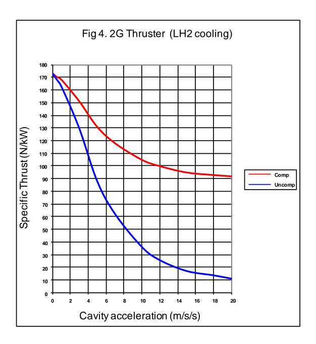
Fig 4 gives the results for a lower frequency cavity cooled by liquid Hydrogen, thus operating at a temperature of 20deg K, and achieving a static specific thrust of 173 N/kW, with an unloaded Q factor of 3.9x10<sup>7</sup>.
