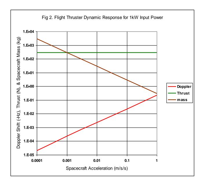
The Dynamic performance of the non superconducting Flight Test model, manufactured and tested by SPR Ltd, and described in REF 3 was modelled with a cavity Qu = 50,000 and  $F_{res}=3.85$  GHz.
