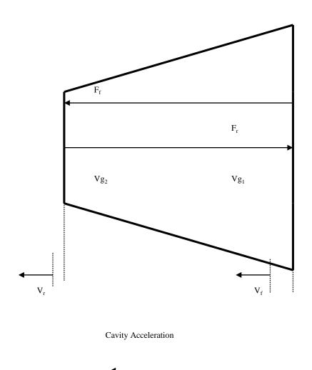
Cavity acceleration produces unequal Doppler Shifts in F<sub>f</sub> and F<sub>r</sub> during each wavefront transit.
