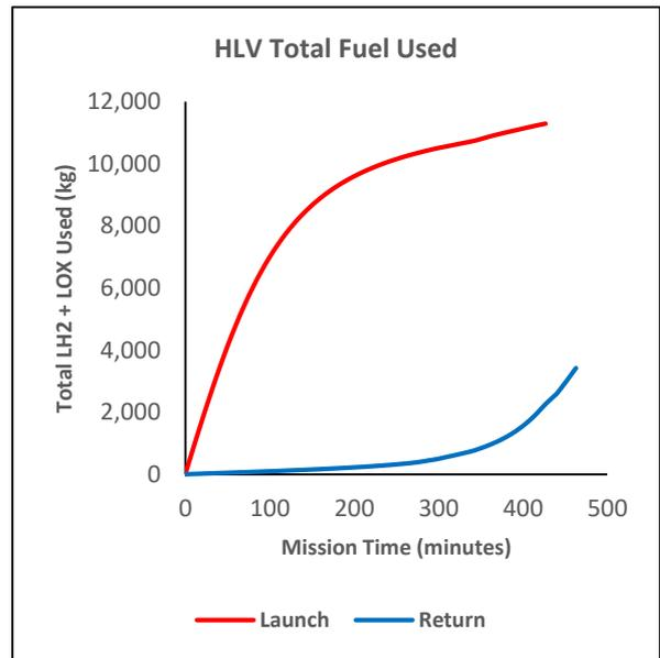
Fig 12. Total LH2 and LOX used for launch and return flights
