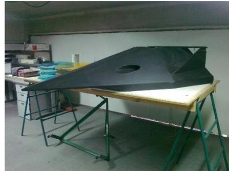
Fig.1. Aerodynamic test model of EmDrive Spaceplane
