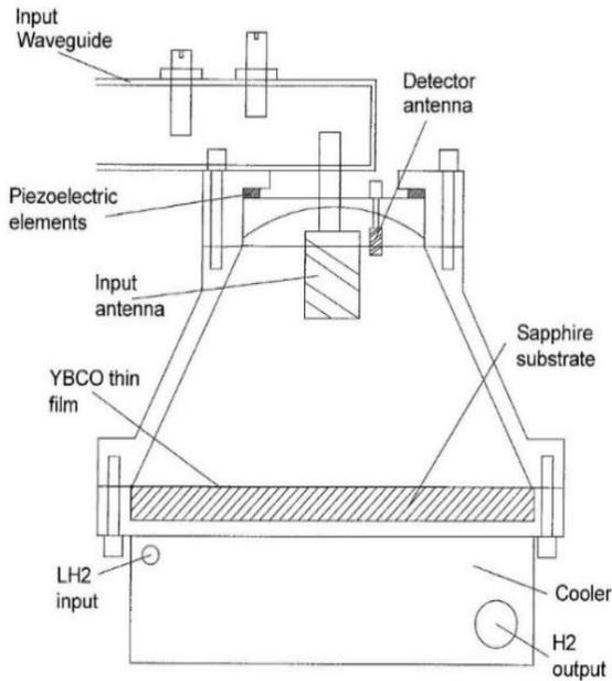
Fig. 4. Superconducting Cavity
