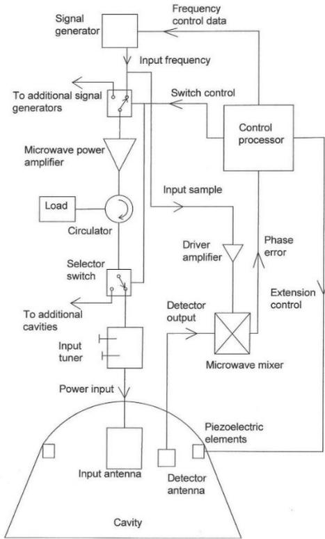
Fig.7. Thruster control system
